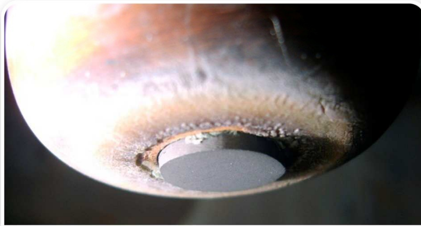
The HfB 2 /SiC sample enshrined in the holder
